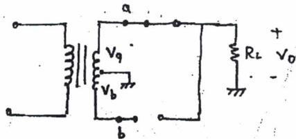
As node a is connected to  $R_L$  so  $V_a$  appears across  $R_L$ .
