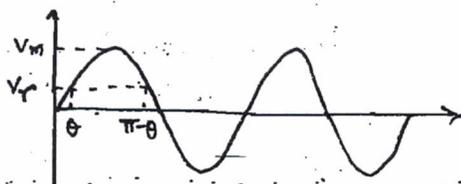
If diode has cut-in voltage  $V_r$  conduction occurs when i/p voltage exceeds cut in voltage therefore a non ideal diode conducts from  $\theta$  to  $\pi - \theta$  and conduction angle becomes  $180^\circ - 2\theta$ .
