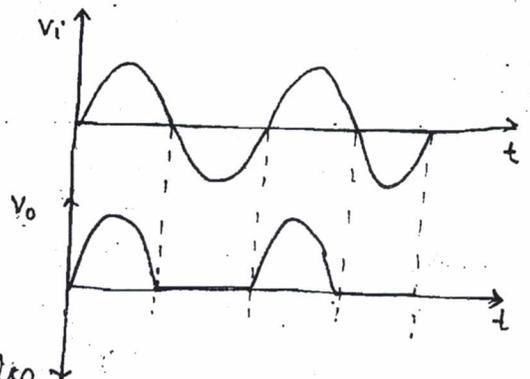
Output waveform is non sinusoidal therefore it also has higher harmonics which can be found in the trigonometric fourier series of  $V_o$ .
