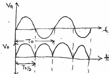
A.C. components has even harmonics i.e.  $2\omega_0, 4\omega_0, 6\omega_0$  etc. It does not have fundamental frequency  $\omega_0$ . Due to this filtering process will be relatively easier in F.W.R
