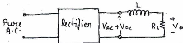
→ For proper filtering operation inductor should be selected such that  $|X_L| \gg R_L$  for half wave rectifier.
