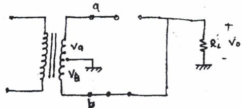
As node b is connected to  $R_L$  so  $V_b$  appears across  $R_L$ .
