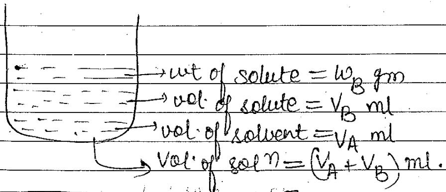
$$\frac{\% w}{V} = \frac{w_B \text{ gm}}{(V_A + V_B) \text{ ml}} \times 100$$
