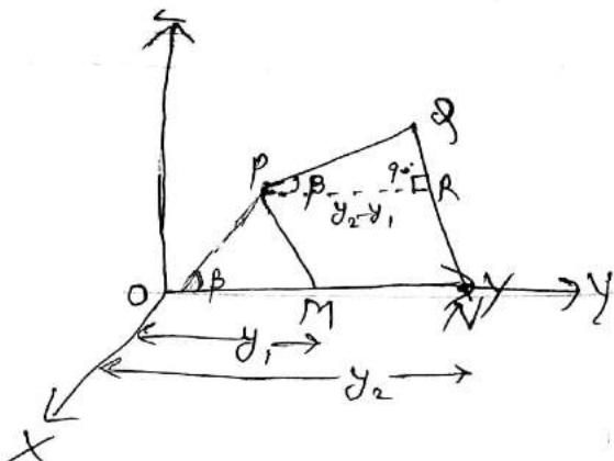
$$\cos \theta = \frac{a_1 a_2 + b_1 b_2 + c_1 c_2}{\sqrt{a_1^2 + b_1^2 + c_1^2} \sqrt{a_2^2 + b_2^2 + c_2^2}}$$
